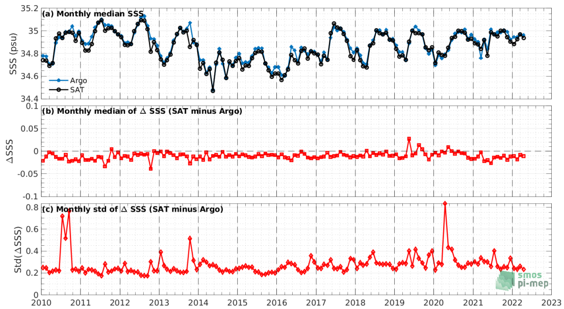
Figure 7: Time series of the monthly median SSS (top), median of \Delta SSS (Satellite - Argo) and Std of \Delta SSS (Satellite - Argo) over the Equatorial Ocean 10N-10S Pi-MEP region considering all match-ups collected by the Pi-MEP.
