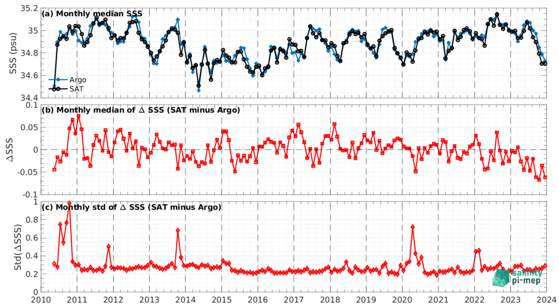
Figure 8: Time series of the monthly median SSS (top), median of \Delta SSS (Satellite - Argo) and Std of \Delta SSS (Satellite - Argo) over the Equatorial Ocean 10N-10S Pi-MEP region considering all match-ups collected by the Pi-MEP.
