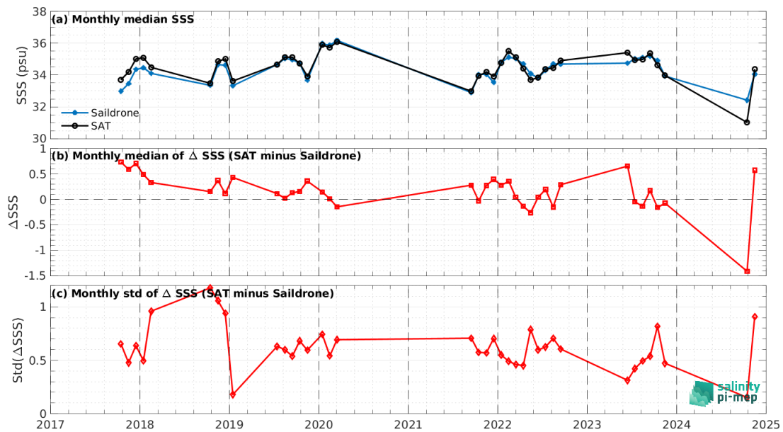
Figure 8: Time series of the monthly median SSS (top), median of \Delta SSS (Satellite - Saildrone) and Std of \Delta SSS (Satellite - Saildrone) over the Equatorial Ocean 10N-10S Pi-MEP region considering all match-ups collected by the Pi-MEP.
