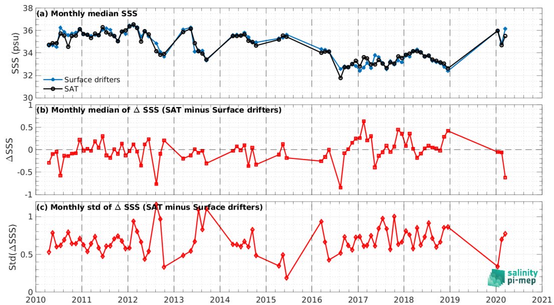
Figure 7: Time series of the monthly median SSS (top), median of \Delta SSS (Satellite - Surface drifters) and Std of \Delta SSS (Satellite - Surface drifters) over the Equatorial Ocean 10N-10S Pi-MEP region considering all match-ups collected by the Pi-MEP.
