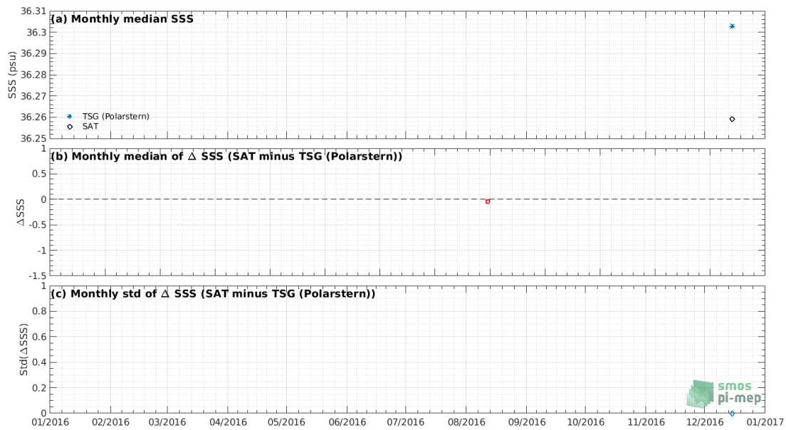
Figure 7: Time series of the monthly median SSS (top), median of \Delta SSS (Satellite - TSG (Polarstern)) and Std of \Delta SSS (Satellite - TSG (Polarstern)) over the Congo river plume Pi-MEP region considering all match-ups collected by the Pi-MEP.
