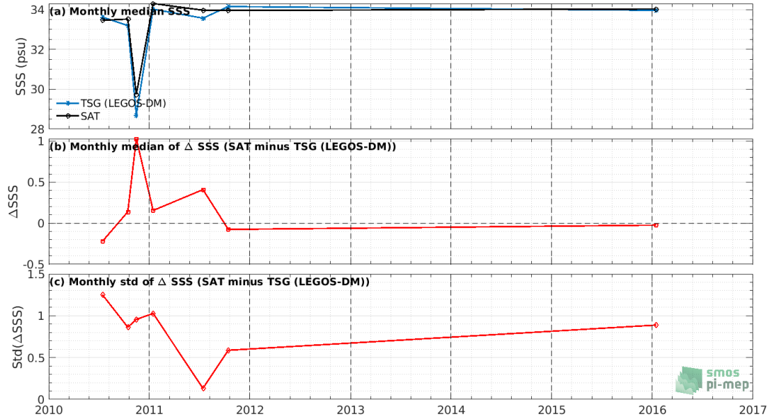
Figure 7: Time series of the monthly median SSS (top), median of \Delta\text{SSS} (Satellite - TSG (LEGOS-DM)) and Std of \Delta\text{SSS} (Satellite - TSG (LEGOS-DM)) over the Bay of Bengal Pi-MEP region considering all match-ups collected by the Pi-MEP.
