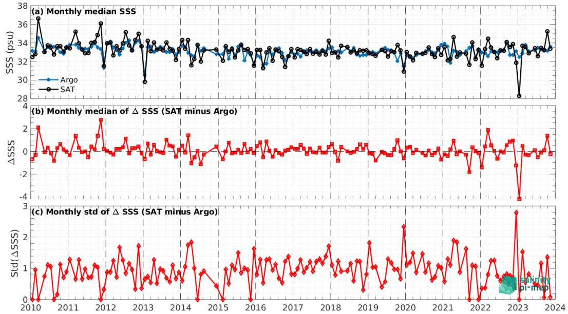
Figure 8: Time series of the monthly median SSS (top), median of \Delta SSS (Satellite - Argo) and Std of \Delta SSS (Satellite - Argo) over the Bay of Bengal Pi-MEP region considering all match-ups collected by the Pi-MEP.
