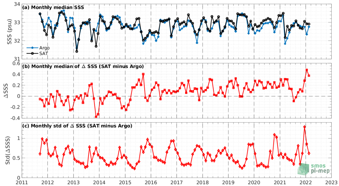
Figure 7: Time series of the monthly median SSS (top), median of \Delta SSS (Satellite - Argo) and Std of \Delta SSS (Satellite - Argo) over the Bay of Bengal Pi-MEP region considering all match-ups collected by the Pi-MEP.
