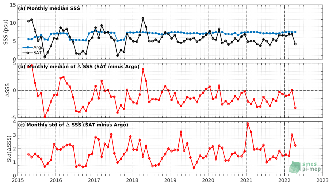
Figure 7: Time series of the monthly median SSS (top), median of \Delta SSS (Satellite - Argo) and Std of \Delta SSS (Satellite - Argo) over the Baltic Sea Pi-MEP region considering all match-ups collected by the Pi-MEP.
