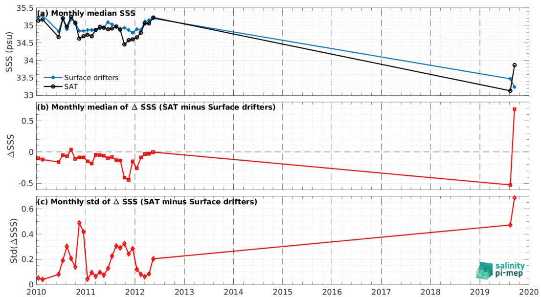
Figure 6: Time series of the monthly median SSS (top), median of \Delta SSS (Satellite - Surface drifters) and Std of \Delta SSS (Satellite - Surface drifters) over the Arctic Ocean Pi-MEP region considering all match-ups collected by the Pi-MEP.
