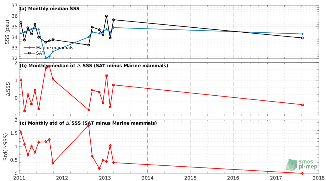
Figure 7: Time series of the monthly median SSS (top), median of \Delta SSS (Satellite - Marine mammals) and Std of \Delta SSS (Satellite - Marine mammals) over the Arctic Ocean Pi-MEP region considering all match-ups collected by the Pi-MEP.
