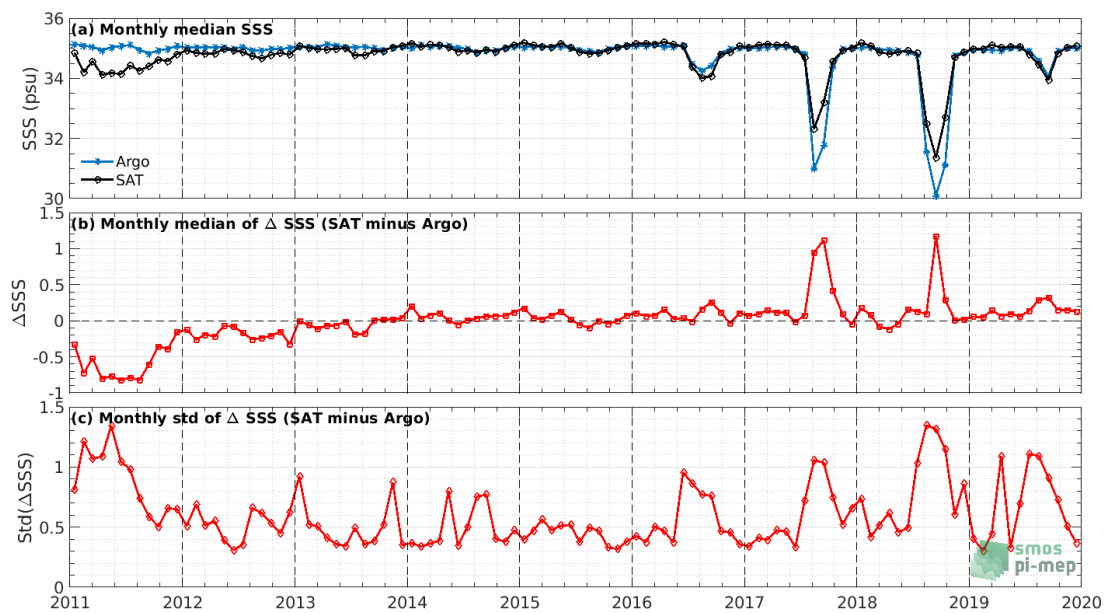
Figure 7: Time series of the monthly median SSS (top), median of \Delta SSS (Satellite - Argo) and Std of \Delta SSS (Satellite - Argo) over the Arctic Ocean Pi-MEP region considering all match-ups collected by the Pi-MEP.
