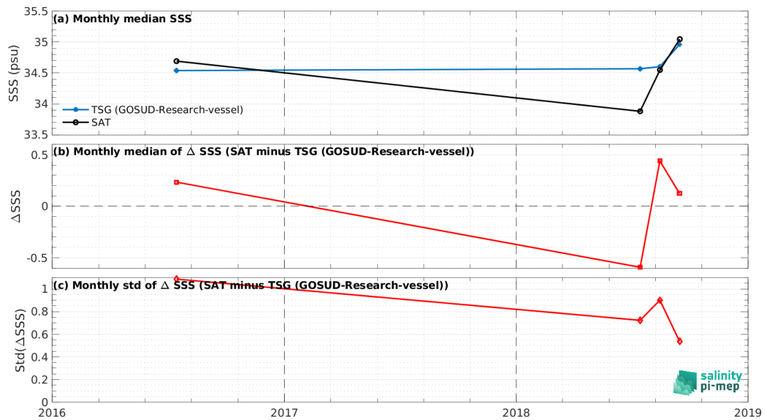
Figure 8: Time series of the monthly median SSS (top), median of \Delta SSS (Satellite - TSG (GOSUD-Research-vessel)) and Std of \Delta SSS (Satellite - TSG (GOSUD-Research-vessel)) over the Arctic Ocean Pi-MEP region considering all match-ups collected by the Pi-MEP.
