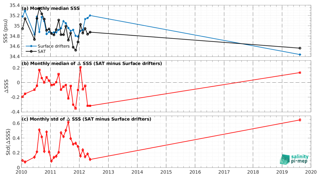
Figure 7: Time series of the monthly median SSS (top), median of \Delta SSS (Satellite - Surface drifters) and Std of \Delta SSS (Satellite - Surface drifters) over the Arctic Ocean Pi-MEP region considering all match-ups collected by the Pi-MEP.
