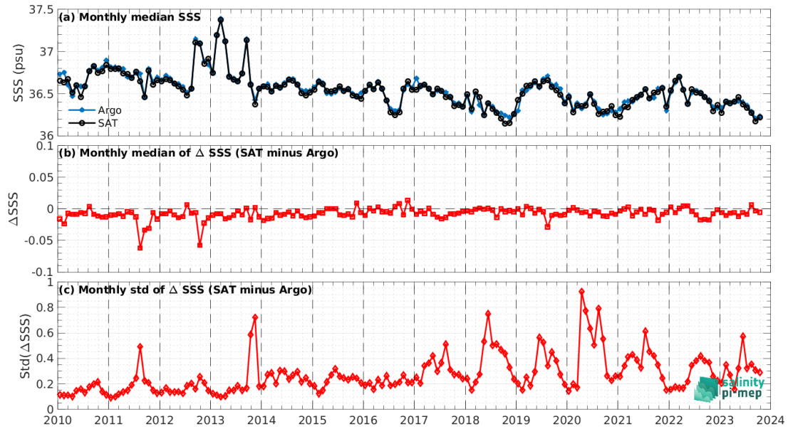
Figure 7: Time series of the monthly median SSS (top), median of \Delta SSS (Satellite - Argo) and Std of \Delta SSS (Satellite - Argo) over the Amazon and Orinoco river plumes Pi-MEP region considering all match-ups collected by the Pi-MEP.
