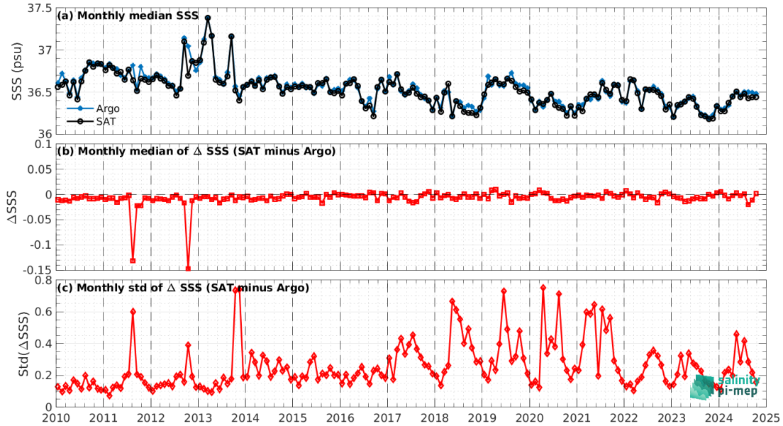
Figure 8: Time series of the monthly median SSS (top), median of \Delta SSS (Satellite - Argo) and Std of \Delta SSS (Satellite - Argo) over the Amazon and Orinoco river plumes Pi-MEP region considering all match-ups collected by the Pi-MEP.
