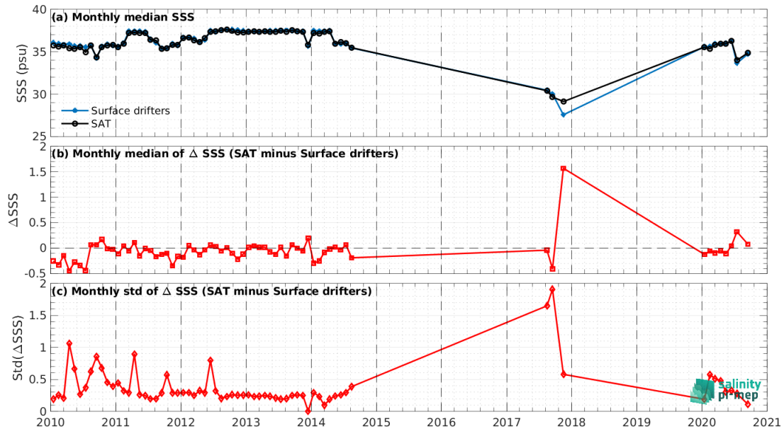
Figure 7: Time series of the monthly median SSS (top), median of \Delta\text{SSS} (Satellite - Surface drifters) and Std of \Delta\text{SSS} (Satellite - Surface drifters) over the Amazon and Orinoco river plumes Pi-MEP region considering all match-ups collected by the Pi-MEP.
