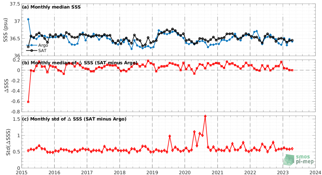
Figure 7: Time series of the monthly median SSS (top), median of \Delta\text{SSS} (Satellite - Argo) and Std of \Delta\text{SSS} (Satellite - Argo) over the Amazon and Orinoco river plumes Pi-MEP region considering all match-ups collected by the Pi-MEP.
