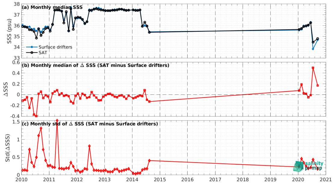
Figure 7: Time series of the monthly median SSS (top), median of \Delta SSS (Satellite - Surface drifters) and Std of \Delta SSS (Satellite - Surface drifters) over the Amazon and Orinoco river plumes Pi-MEP region considering all match-ups collected by the Pi-MEP.
