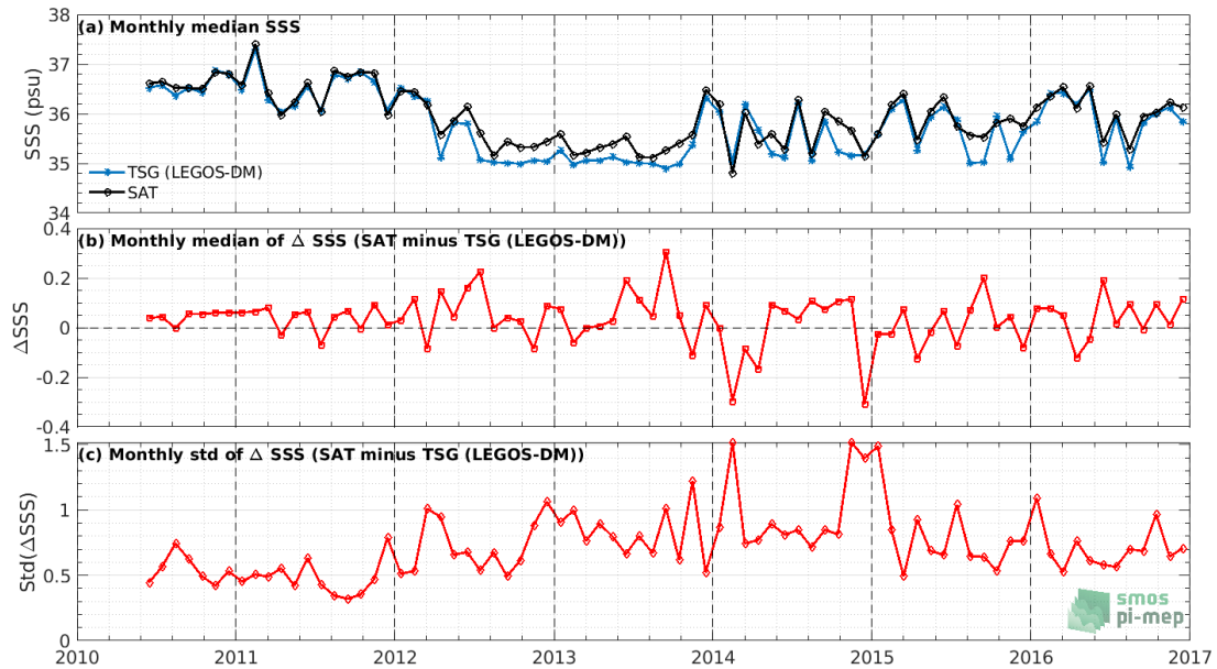
Figure 7: Time series of the monthly median SSS (top), median of \Delta SSS (Satellite - TSG (LEGOS-DM)) and Std of \Delta SSS (Satellite - TSG (LEGOS-DM)) over the Atlantic Ocean Pi-MEP region considering all match-ups collected by the Pi-MEP.
