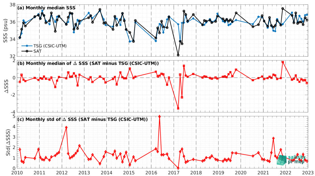
Figure 7: Time series of the monthly median SSS (top), median of \Delta SSS (Satellite - TSG (CSIC-UTM)) and Std of \Delta SSS (Satellite - TSG (CSIC-UTM)) over the Atlantic Ocean Pi-MEP region considering all match-ups collected by the Pi-MEP.
