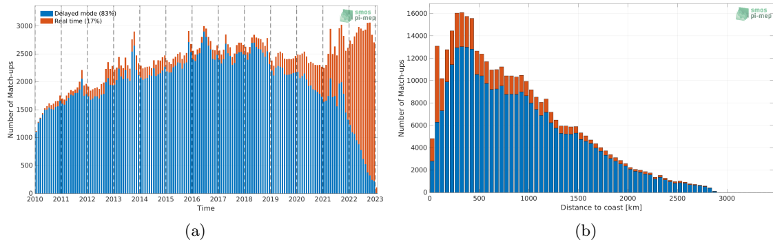
Figure 1: Number of match-ups between Argo and SMOS SSS L3 v8 - 9 Days (CATDS-CECOS-LOCEAN) SSS as a function of time (a) and as function of the distance to coast (b) over the Atlantic Ocean Pi-MEP region and for the full satellite product period.
