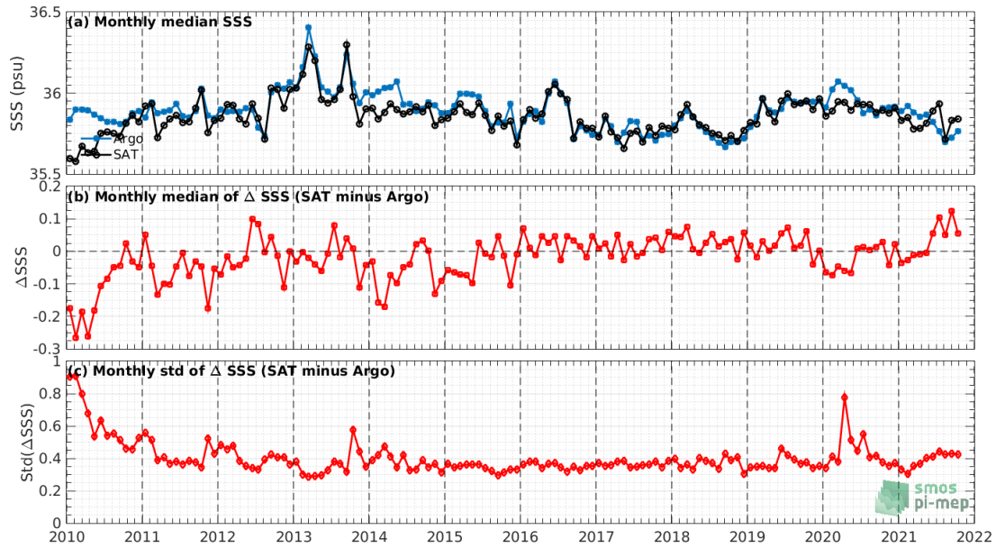
Figure 7: Time series of the monthly median SSS (top), median of \Delta SSS (Satellite - Argo) and Std of \Delta SSS (Satellite - Argo) over the Atlantic Ocean Pi-MEP region considering all match-ups collected by the Pi-MEP.
