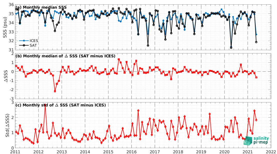
Figure 8: Time series of the monthly median SSS (top), median of \Delta SSS (Satellite - ICES) and Std of \Delta SSS (Satellite - ICES) over the Atlantic Ocean Pi-MEP region considering all match-ups collected by the Pi-MEP.
