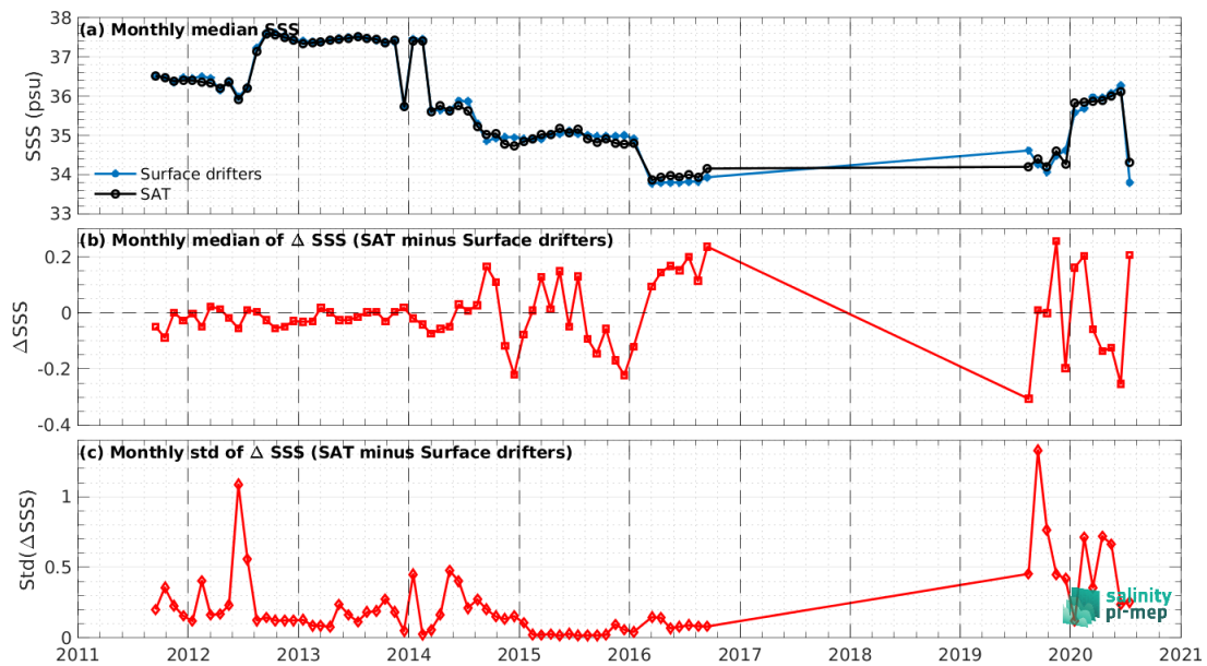
Figure 6: Time series of the monthly median SSS (top), median of \Delta SSS (Satellite - Surface drifters) and Std of \Delta SSS (Satellite - Surface drifters) over the Atlantic Ocean Pi-MEP region considering all match-ups collected by the Pi-MEP.
