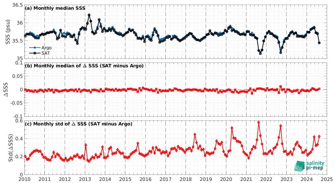
Figure 8: Time series of the monthly median SSS (top), median of \Delta SSS (Satellite - Argo) and Std of \Delta SSS (Satellite - Argo) over the Atlantic Ocean Pi-MEP region considering all match-ups collected by the Pi-MEP.
