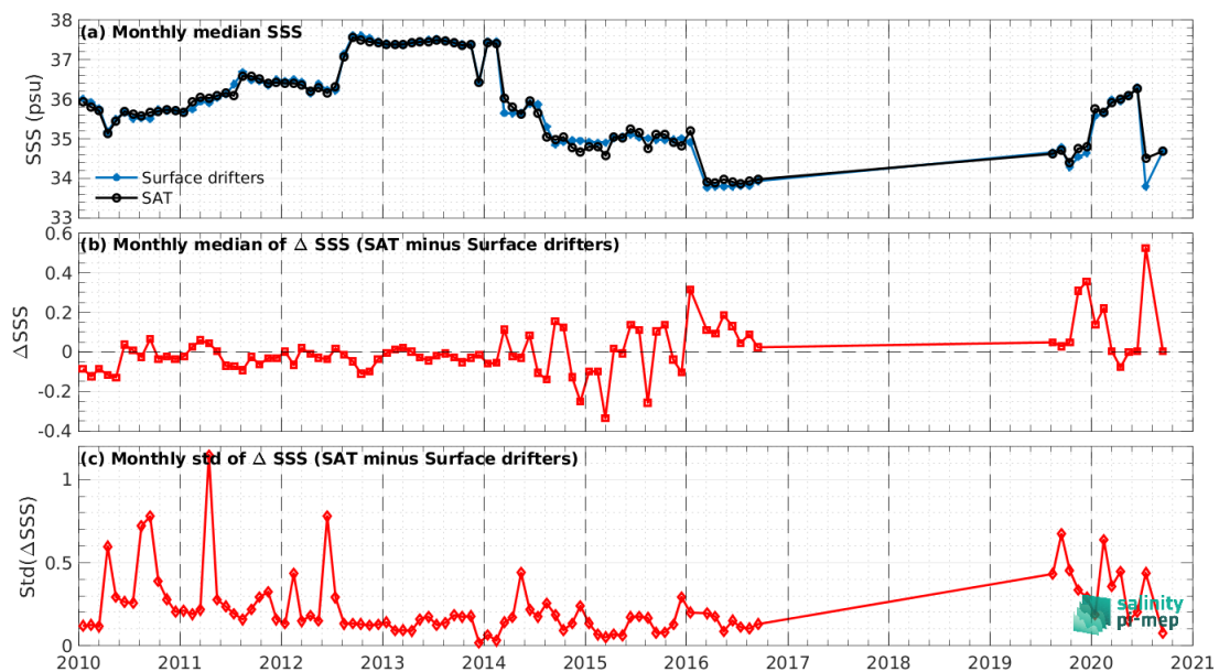
Figure 7: Time series of the monthly median SSS (top), median of \Delta SSS (Satellite - Surface drifters) and Std of \Delta SSS (Satellite - Surface drifters) over the Atlantic Ocean Pi-MEP region considering all match-ups collected by the Pi-MEP.
