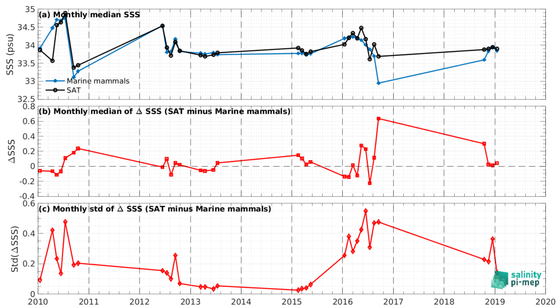
Figure 7: Time series of the monthly median SSS (top), median of \Delta SSS (Satellite - Marine mammals) and Std of \Delta SSS (Satellite - Marine mammals) over the Atlantic Ocean Pi-MEP region considering all match-ups collected by the Pi-MEP.
