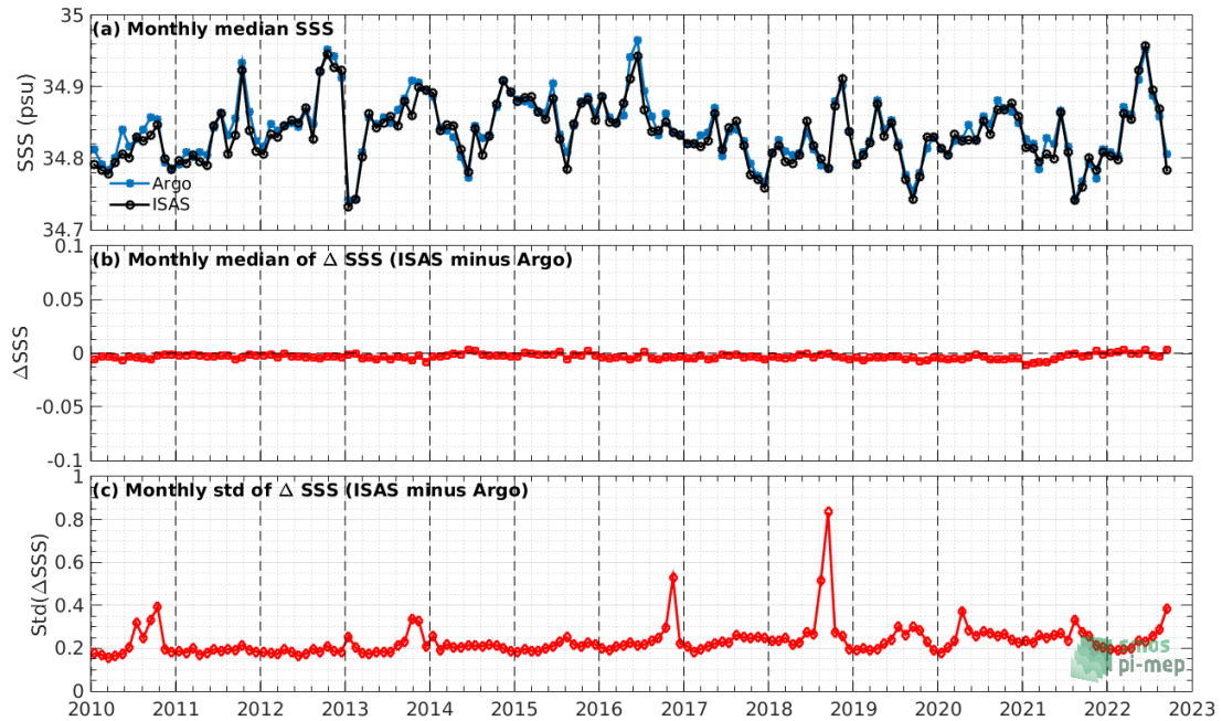
Figure 6: Time series of the monthly median SSS (top), median of \Delta SSS (ISAS - Argo) and Std of \Delta SSS (ISAS - Argo) considering all match-ups collected by the Pi-MEP.
