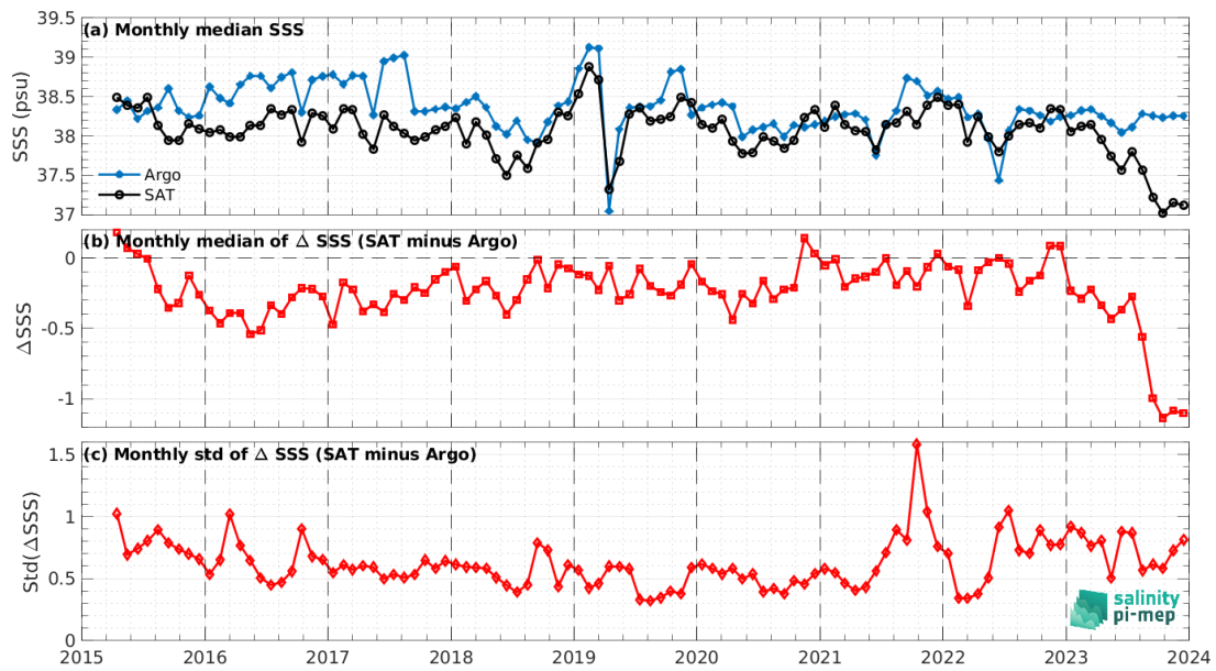
Figure 8: Time series of the monthly median SSS (top), median of \Delta SSS (Satellite - Argo) and Std of \Delta SSS (Satellite - Argo) over the Mediterranean Sea Pi-MEP region considering all match-ups collected by the Pi-MEP.
