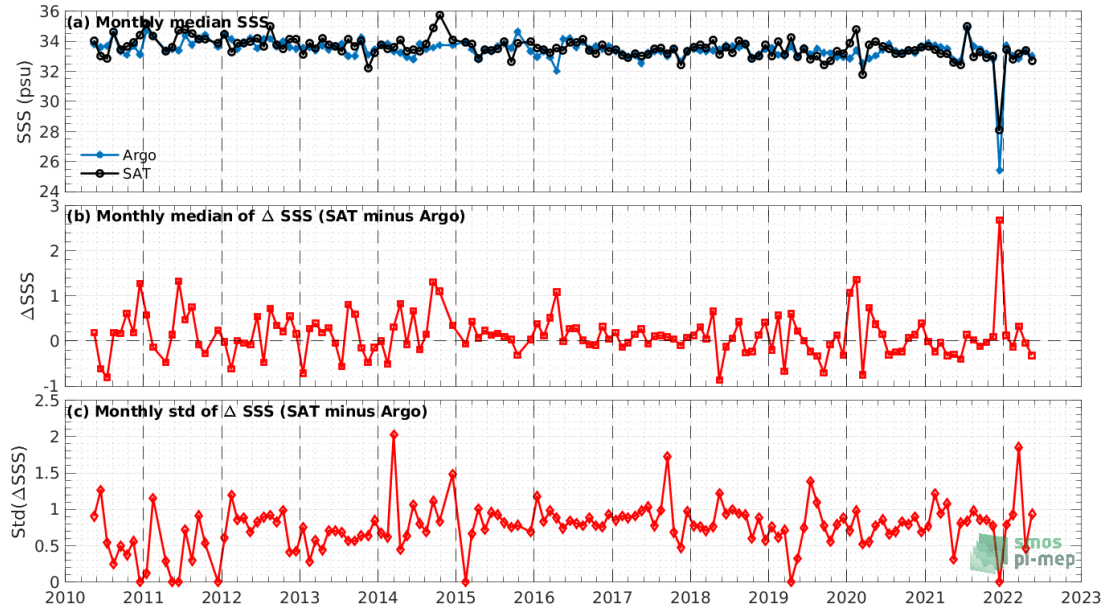
Figure 7: Time series of the monthly median SSS (top), median of \Delta\text{SSS} (Satellite - Argo) and Std of \Delta\text{SSS} (Satellite - Argo) over the Ganga and Brahmaputra river plumes Pi-MEP region considering all match-ups collected by the Pi-MEP.
