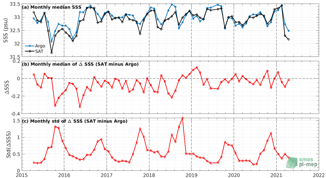
Figure 7: Time series of the monthly median SSS (top), median of \Delta SSS (Satellite - Argo) and Std of \Delta SSS (Satellite - Argo) over the Ganga and Brahmaputra river plumes Pi-MEP region considering all match-ups collected by the Pi-MEP.
