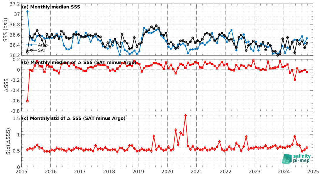
Figure 8: Time series of the monthly median SSS (top), median of \Delta\text{SSS} (Satellite - Argo) and Std of \Delta\text{SSS} (Satellite - Argo) over the Amazon and Orinoco river plumes Pi-MEP region considering all match-ups collected by the Pi-MEP.
