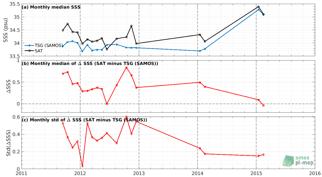
Figure 7: Time series of the monthly median SSS (top), median of \Delta SSS (Satellite - TSG (SAMOS)) and Std of \Delta SSS (Satellite - TSG (SAMOS)) over the Roaring Forties and Furious Fifties Pi-MEP region considering all match-ups collected by the Pi-MEP.
