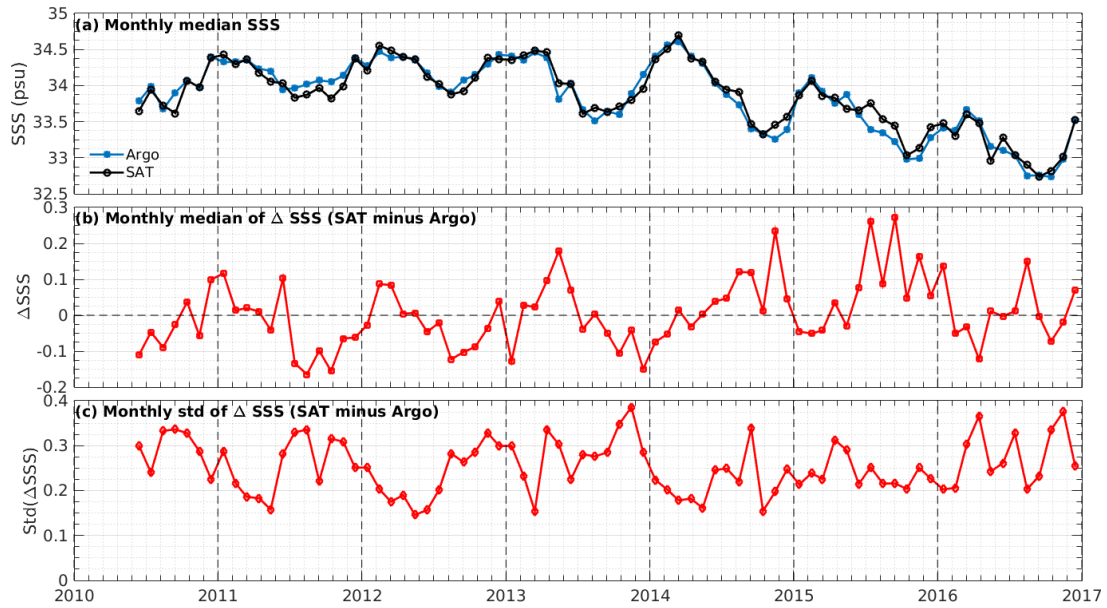
Figure 7: Time series of the monthly median SSS (top), median of \Delta SSS (Satellite - Argo) and Std of \Delta SSS (Satellite - Argo) over the SPURS 2 Pi-MEP region considering all match-ups collected by the Pi-MEP.
