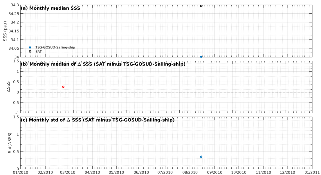
Figure 7: Time series of the monthly median SSS (top), median of \Delta SSS (Satellite - TSG-GOSUD-Sailing-ship) and Std of \Delta SSS (Satellite - TSG-GOSUD-Sailing-ship) over the SPURS 2 Pi-MEP region considering all match-ups collected by the Pi-MEP.
