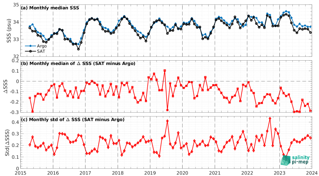
Figure 8: Time series of the monthly median SSS (top), median of \Delta SSS (Satellite - Argo) and Std of \Delta SSS (Satellite - Argo) over the SPURS 2 Pi-MEP region considering all match-ups collected by the Pi-MEP.
